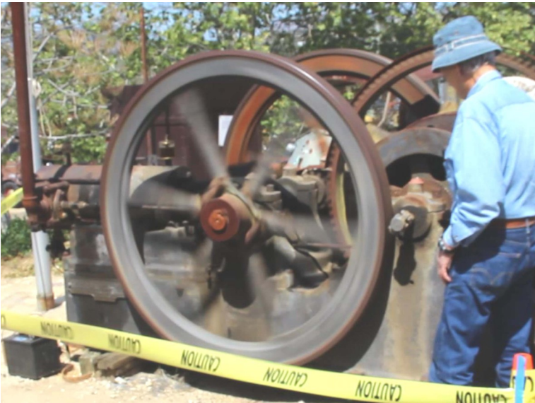
Frank Ball coaxes the 1899 Fairbanks –Morse single cylinder gas engine to life.
